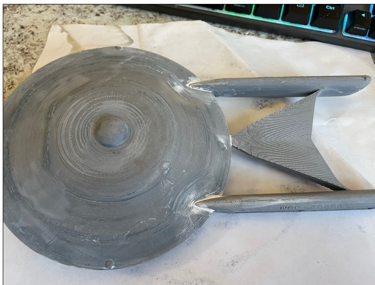
Ship put together, putty (white) applied. And now, more sanding...
