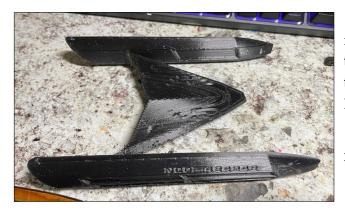
After wondering what in the world to do about it, and running out of filament (which ain't cheap, I can tell you!) I put it back out in the sun to soften, and then molded it back into shape over the last saucer-top I'd made. Worked well.
